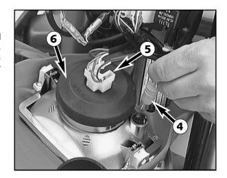
Insert the new lamp such that the noses (7) engage in the recesses (8). When doing so, do not touch the glass body of the lamp so that it remains free from fat. Engage retaining clip, mount rubber cap and connector. If the parking-light lamp is to be replaced, simply insert it in the holder. Reinsert the parking-light lamp together with the holder.
