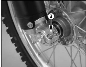
To install the front wheel, lift it into the fork, position and mount the axle shaft (4). Mount the collar nut (2), tighten the clamping screws (3) on the right fork leg axle passage to prevent the axle shaft from turning and tighten the collar nut to 40 Nm.
