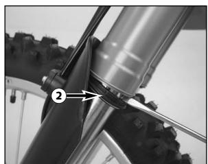
Clean the dust-protection bellows, outer tubes, and fork tubes thoroughly, and oil them thoroughly with silicone spray or engine oil. Then, push the dust-protection bellows into the outer tubes by hand.
