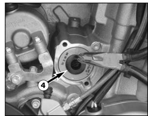
Lay the motorcycle down and fill the oil filter housing approx. half-full with engine oil. Insert the oil filter in the housing. Grease the O-rings in the oil filter cover and mount the cover. Mount the screws and tighten to 6 Nm.
