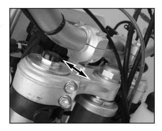
For this purpose, remove screws (3) of the handlebar clamps and screws (4) of the handlebar support. Position the handlebar support, and tighten screws (4) to 40 Nm. Mount handlebar and handlebar clamps, and tighten screws (3) to 20 Nm. The gap between the handlebar support and the handlebar clamps should be the same in the front and in the rear.
